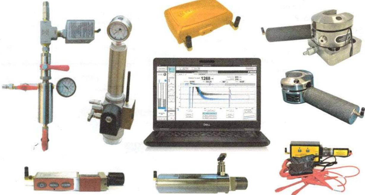
Wireless sensor set up and installation is done efficiently by using the control buttons and LED displays, mounted on the sensor's body, which are used to power up, adjust, and calibrate the sensors when installed at the wellhead without having to view the computer screen.
